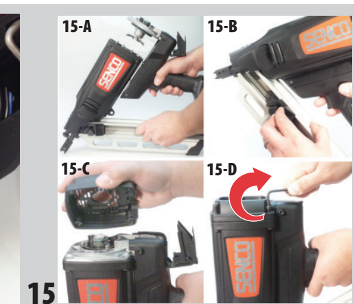
15 Reinstall Flange Assembly. Place Flange Assembly on top of Combustion Chamber. Pull Feeder Shoe back, depress Safety and hold in position. Reinstall Top Cover with 4 Screws and tighten. (Failure to fully depress Safety before tightening Top Cover Screws will cause O-Ring on Flange Assembly to become damaged)
