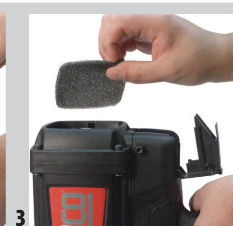
3 Remove and discard Filter.
