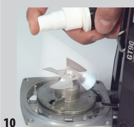
10 Spray with Tool Cleaner (PC1235) and wipe off with a clean dry cloth.
