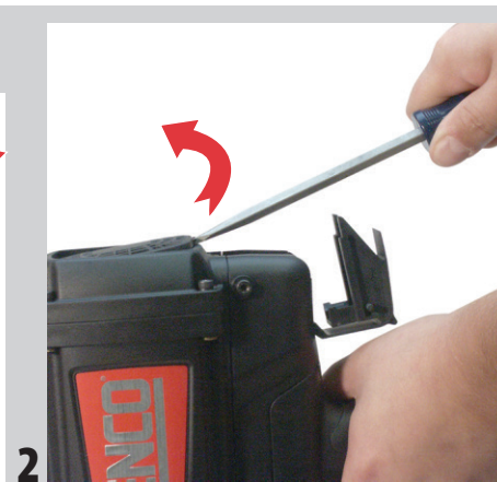
2 Remove Filter Cover with a flat blade screw driver.
