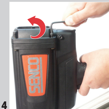
4 Remove 4 Cap Screws and Washers (4mm Allen Wrench).
