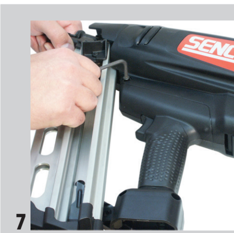
7 Remove Screw and Washer from Anti-Rotation Screw (4mm Allen Wrench). Slide the Anti-Rotation Screw out the other side.
