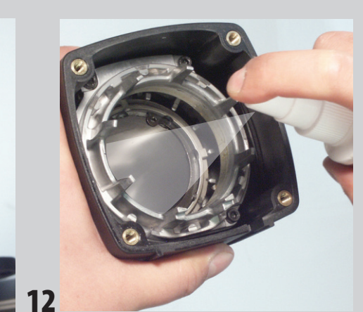
12 Apply Tool Cleaner (PC1235) into Combustion Chamber and Cylinder Sleeve area (some cleaner may leak out bottom vent area of tool). Wipe out with a clean dry cloth.
