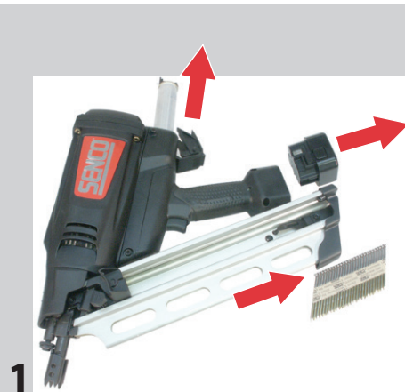
1 Remove Fasteners, Battery and Fuel Cell.
