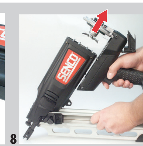
8 Remove Handle (Includes Top Flange Assembly). Pull Handle Back over Flange on Main Body Housing, lift straight up BEING CAREFUL NOT TO DAMAGE FAN.
