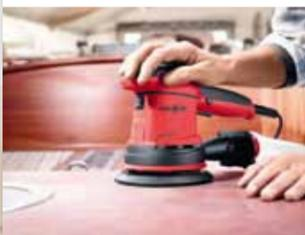
For fine sanding and when sanding between coats, a stroke of 3 mm makes the EVA 150 E/3 particularly adept.
