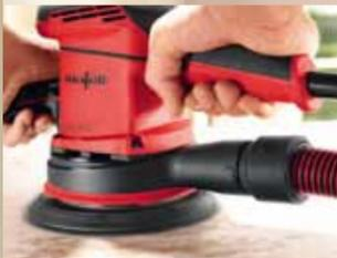
In combination with an efficient dust extractor, the large number of suction channels remove as much dust as possible. Even without a separate dust extraction system attached to the machine, the EVA 150 E operates very efficiently and generates very little dust thanks to its powerful extraction turbine.
