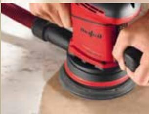
The EVA 150 E offers a 20 percent higher speed than conventional random orbital sanders, which appreciably increases the removal rate. As a result, given the same quality of surface, you can perform the work up to 20 percent quicker and ultimately save costs.
